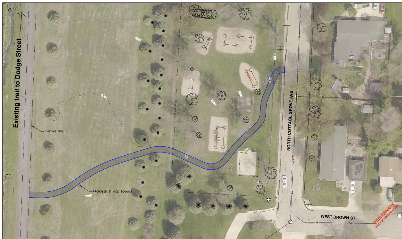
The Hawkinson Park Trail Connection project includes construction of an 8-foot-wide concrete trail that provides handicap access from Cottage Grove Avenue into Hawkinson Park and connects to the Luverne Loop Trail.
