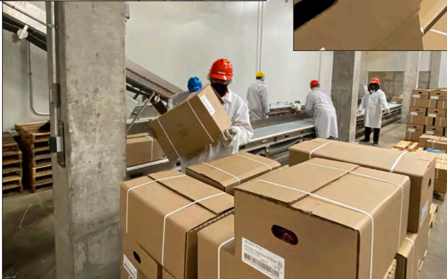
From the cut floor, product is labeled, palletized and either loaded on refrigerated semitrailers or sent to the packaging area for bagging, cryovacs and box packing before shipping out.
