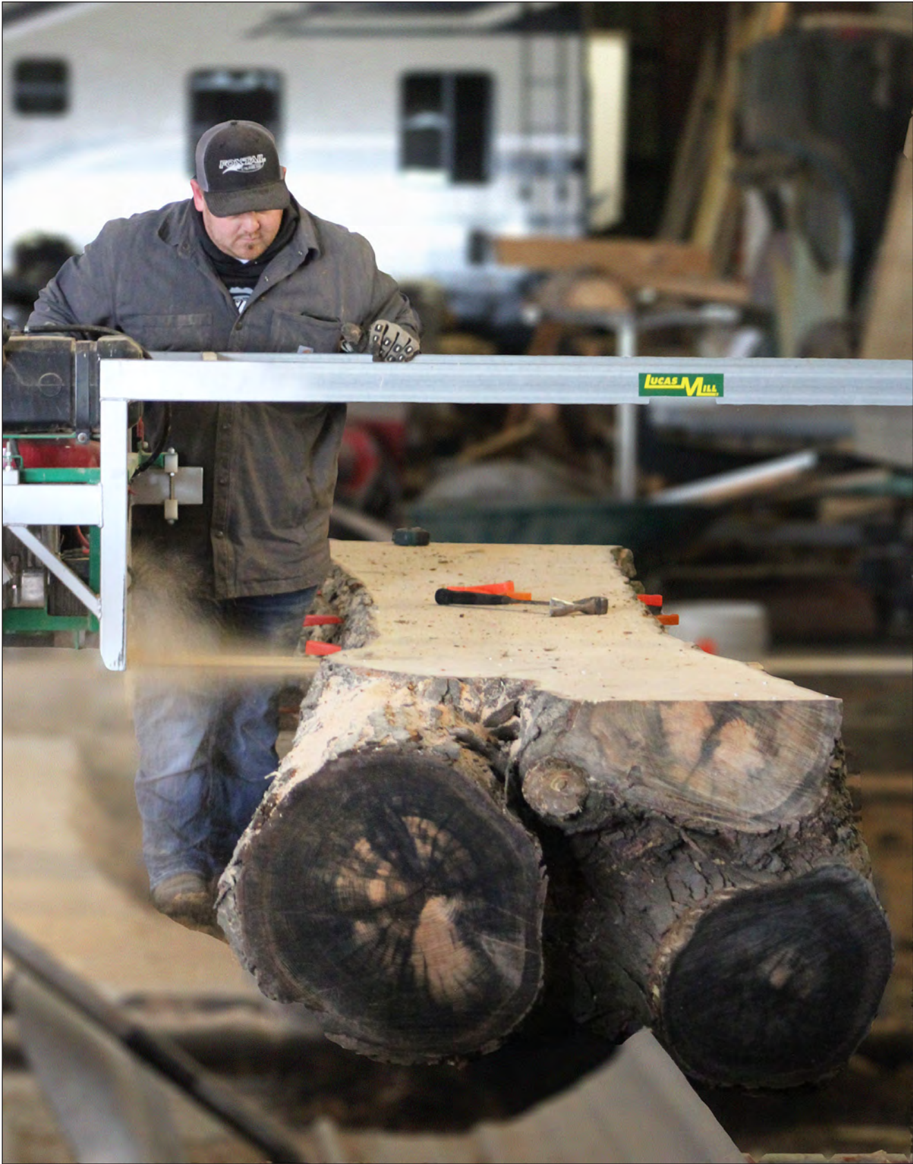
Saw dust is discharged by the Lucas mill’s chain saw as Ryan Bullerman moves the saw through the log. Mavis Fodness photo/0401 Home Tab 2021 Bullys
